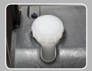
Brake fluid reservoir with level switch
